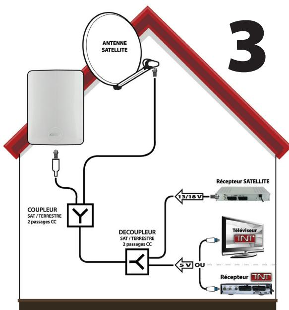
This plan represents an installation combining at the same time a terrestrial reception and a satellite reception. Both antennas are then connected by a mixer (with 2 passages of current). To redistribute the signals, it will be necessary to use a case to demixer (with 2 passages of current). Quite as in the case n°1, the supply of the antenna will be made by the device of reception.
