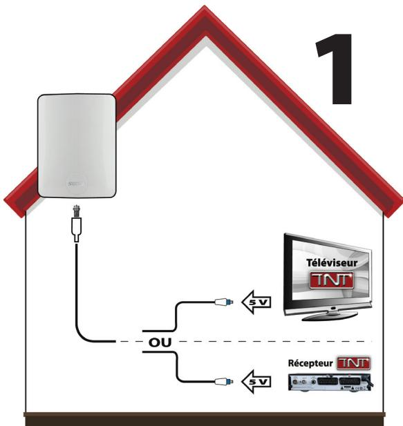
In this case, the antenna is connected directly on the receiver TNT or the television set. The power necessary (5 Volts) is then provided by the receiver or the television set by activating this function in the menu. The injector is not essential in this installation, it can any time being used without connecting it to the sector like attenuator of signal (potentiometer)
