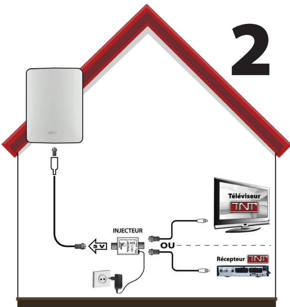
Here, the injector of tension will be used (not function power antenna in the receiver or television set TNT). The injector is then connected between the antenna and the device of reception. This one is also connected to a power-socket using the adapter.
