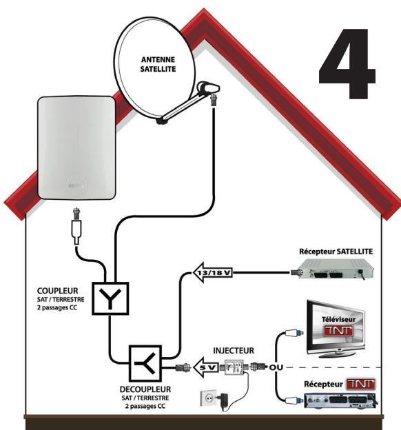
Here, the injector of tension will be used (not function power antenna in the receiver or television set TNT). The injector is thus connected between the TERRESTRIAL output of the demixer and the device of reception. This one is also connected to a power-socket using the adapter.
