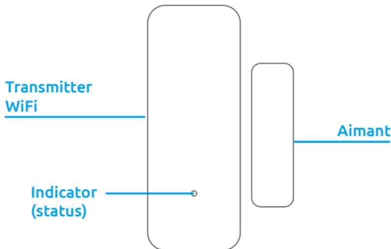
The WiFi opening detector allows you to be alerted when your door or window is open. This device can have several uses: it improves the security of your home, it can allow you to monitor the different openings of accesses (to check if your child is home from school for example). Associated with other connected objects, the WiFi opening detector can also trigger scenarios (e.g. activation of the light when the front door is opened after a certain time...).
