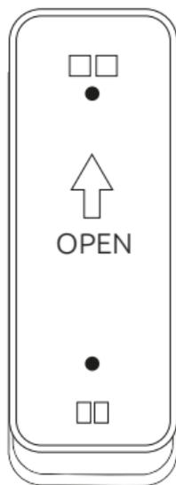
Push the back cover of the transmitter up to access the battery compartment.
