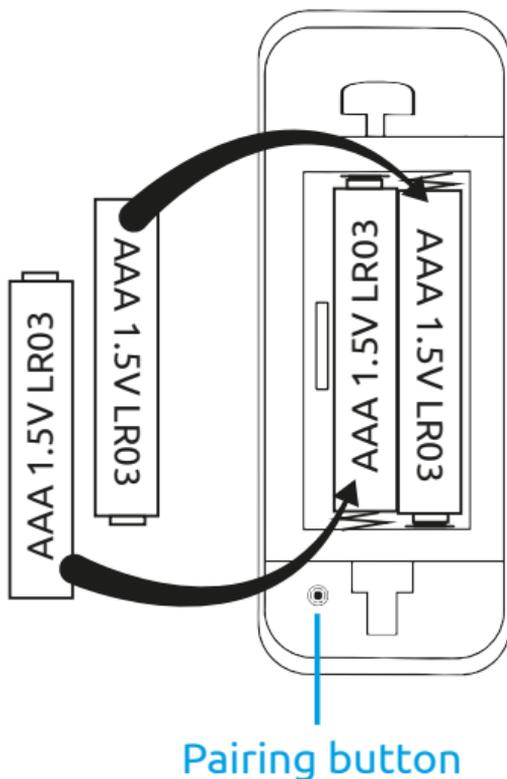
Insert 2 AAA 1.5 volt batteries (LR03) into the battery compartment, observing the correct polarity.
