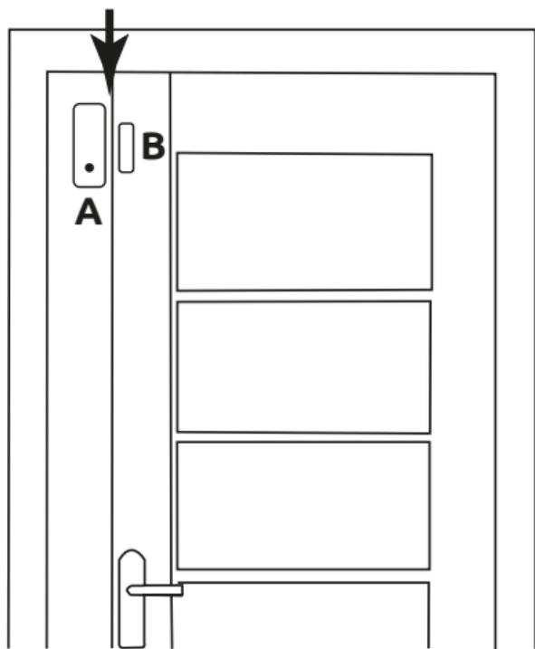
If the support allows it (e.g. wooden door), you can use screws (not supplied) to fix the transmitter and its magnet.
