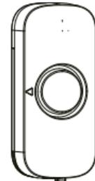
4. Peel the sticker off the magnet, then stick it to the moving part of your door or window. Make sure that the arrows are aligned and that the gap between the 2 elements is less than 20 mm. Installation is now complete.
